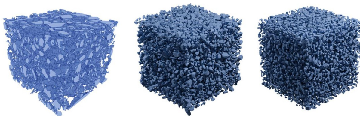
Figure 1: From left to right: an observation of a lithium sulfate particle system, the polyhedral model, the simplified cuboid model. The observation is the result of a SR-nano-CT imaging campaign at the PETRA III beamline P05 at DESY.
